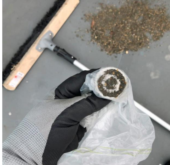
Sweep : Magnetic Screening (80% of cosmic spherules are magnetic) : Bag abt 30g
